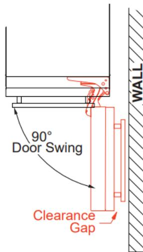
When installing with The hinge side next to a wall - Leave adequate space for your door handle.
