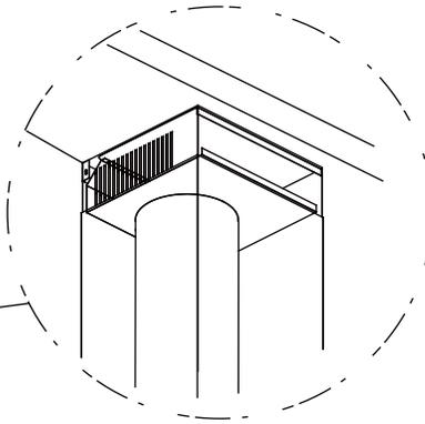
Remove all black foam from filter opening before installing the charcoal filter brackets.
